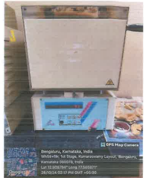
Burnout furnace- to melt wax after investment
