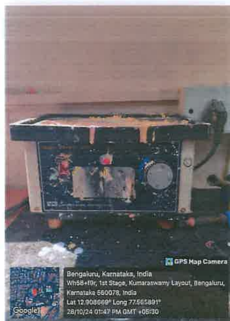
Vibrator- to help in uniform mixing of gypsum and pouring casts.
