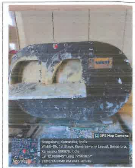
Double Disc Model Trimmer - to trim gypsum models and casts
