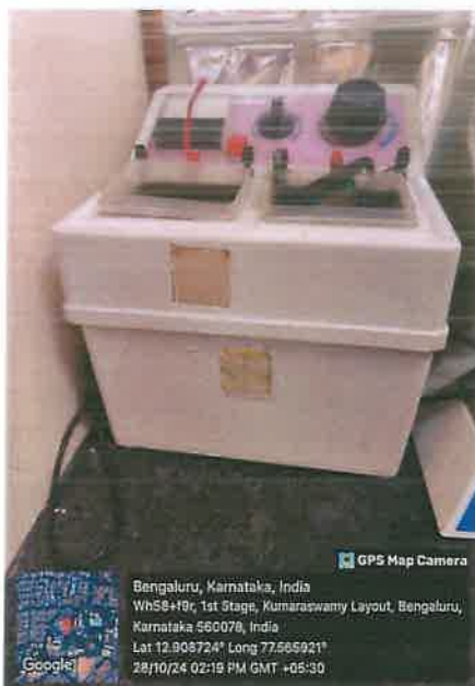
Electro polisher - to polish metal casting electrolytically
